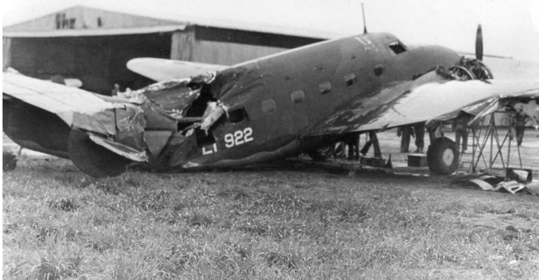
Wreck of the LT922 at Archerfield late February 1942. ML and USAAF personnel are busy taking off the engines to transfer these to aircraft LT919 (Alan Bovelt collection, via Gerard Casius and Gordon Birkett).
